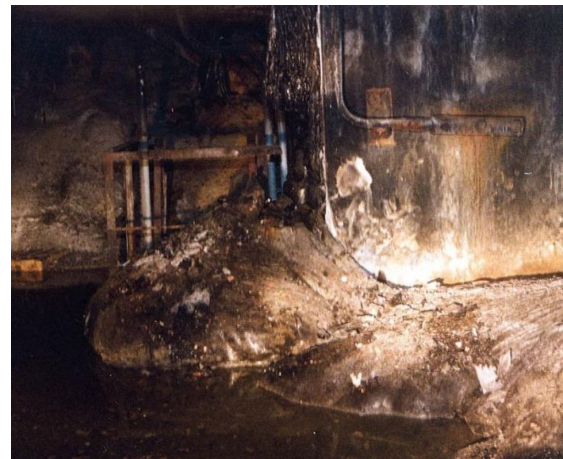
Figure 1.6 – Chernobyl corium found underneath the reactor, also known as the “elephants foot”, in a steam distribution corridor in 1996
