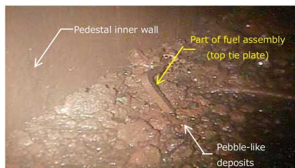
Figure 1.9 – Possible corium "pebble-like" deposits in the primary containment vessel in Fukushima Dai-ichi unit 2
