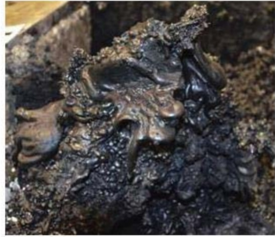
Figure 2.24 – CCI-8 volcanic structure close up showing elongated drop-like, and coalesced particles
