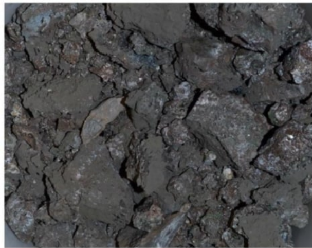
Figure 2.34 – Zoom of a part of the CCI-7 heavily fractured crust found during post-mortem analysis showing the large blocks composing it
