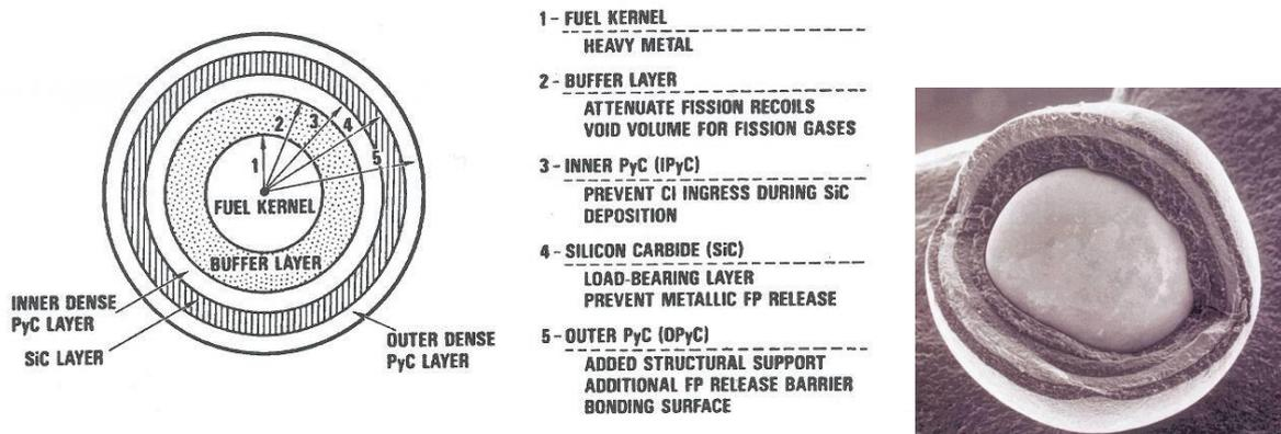
Figure 5: TRISO particles for VHTR
