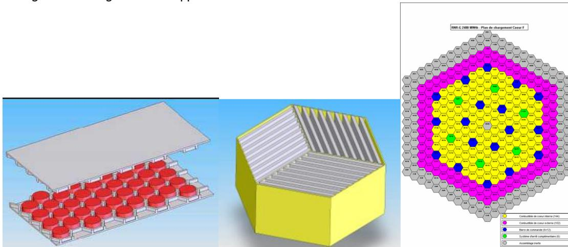
**Figure 3: GFR plate-type fuel and core arrangement**
