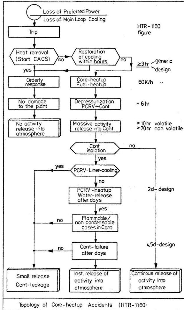
Figure 18: Topology of FP release during core heat-up accidents in VHTRs
