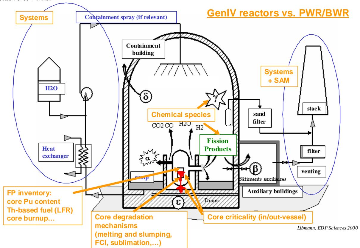
**Figure 14: Containment degradation modes as defined in WASH-1400**
