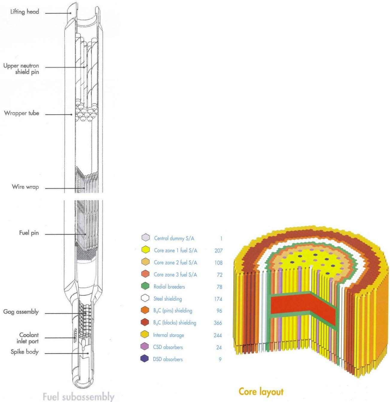
**Figure 2: EFR pin fuel and core arrangement**
