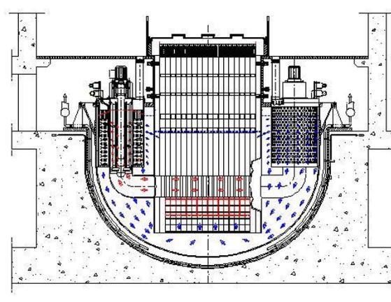
**Figure 9 : sketch of ELSY primary circuit**
