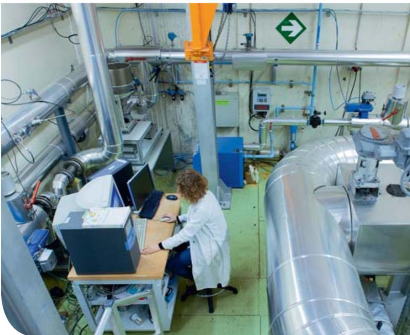
The CATFISH test bench is used to obtain analytical data on HEPA filter clogging.
