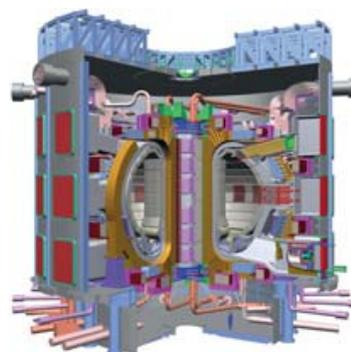
ITER: cross-sectional view of toroidal magnet.
