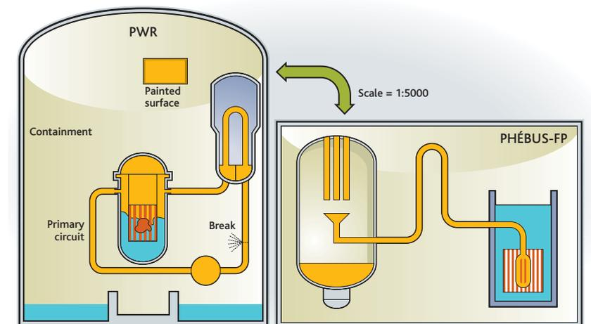
PHEBUS FP facility - a 1:5,000 scale replica of a PWR.
