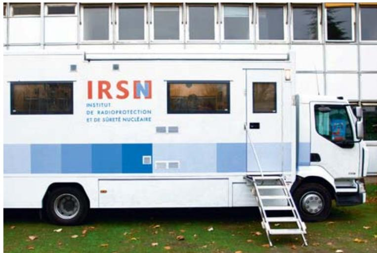
The mobile whole-body counting laboratory is used to monitor worker dosimetry at their workplace.
