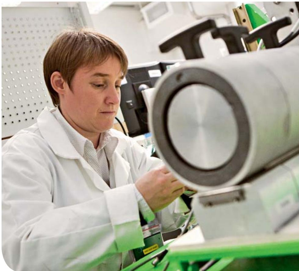
An IRSN engineer tests the gamma spectrometry measuring bench.
