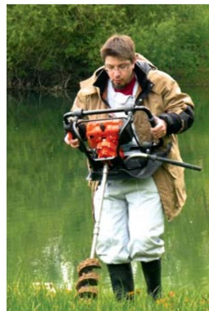
Mechanical auger for soil sampling.
