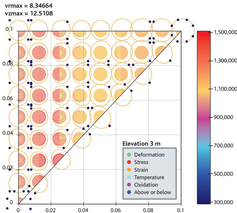
Cross-section of a cluster of fuel rods deformed by a loss-of-coolant accident.
