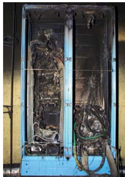
Electrical cabinet after a PICSEL EP test at the DIVA facility.
