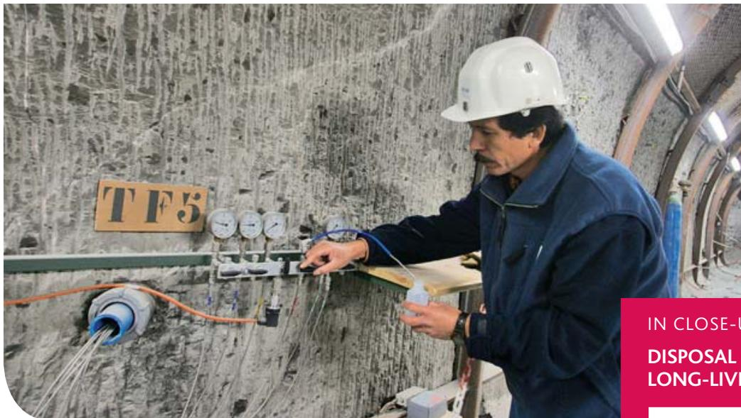
Taking water samples for geochemical analysis at the front of a chemically inert system, isolating a transmissive fracture in the Tournemire experimental station.
