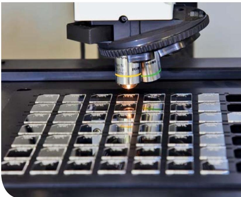
Reading neutron dosimeters.
